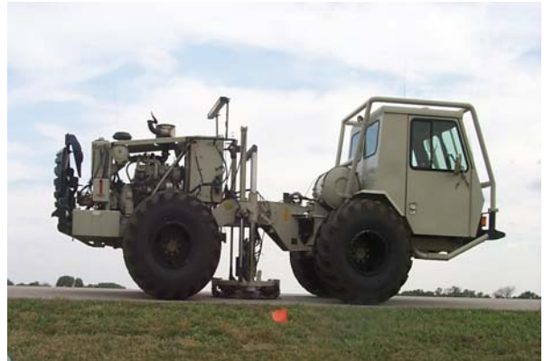
Figure A4. IVI minivib with Atlas rotary valve. Approximately 800 ft-lbs of force can be applied at 100 Hz, while around 2000 ft-lbs are possible in some conditions at 250 Hz.
