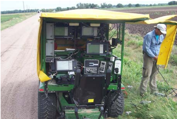
Figure A3. 240 channel Geometrics StrataView with support electronics (line checker, IVI source synchronizer, time break conditioner, etc.).
