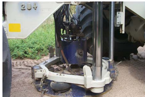
Figure A5. 300 lb mass and 300 lb baseplate with new prototype Atlas rotary valve.
