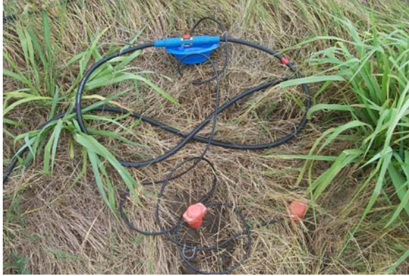
Figure A1. Two Mark Products L28E 40 Hz geophones separated by about 1 ft to form a 2 ft effective array.
