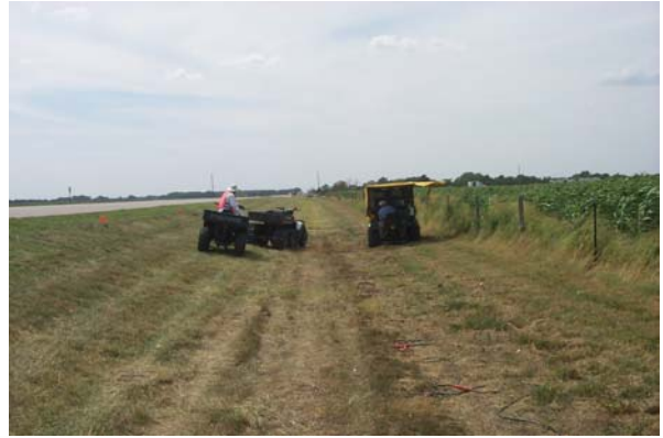
Figure A2. Receivers were "planted" at the base of the road ditch to insure highest possible quality coupling.
