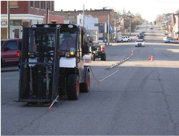
A bungee-assisted weight drop attached to the front of a Bobcat Toolcat (shown here in Galena, Kansas) is one example of active seismic sources used by scientists at the KGS.
