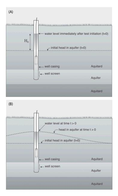
**FIGURE 1.1** Schematic cross sections depicting a slug test in a well screened in a confined aquifer: A) Condition immediately after test initiation; B) Condition some time after initiation (slug test initiated at time t = 0 by rapid insertion of solid object (slug) into the water column, H<sub>0</sub> is the measured initial displacement (water-level change produced by slug insertion), figures not to scale).
