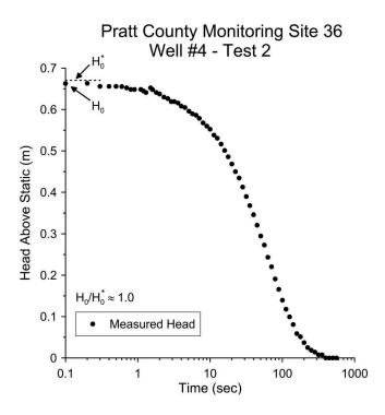
**FIGURE 1.2** Plot of head above static versus log time since test began for a slug test performed in well #4 at monitoring site 36 in Pratt County, Kansas ( $H_0$  is the measured initial displacement in the well and  $H_0^*$  is the expected initial displacement for the test).
