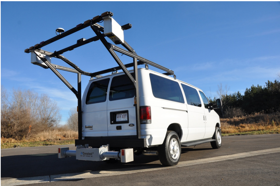
Figure 1— The Pavement Data Collection System van. The boxes mounted on top are the Laser Crack Imaging System cameras that make images of the pavement and elevation measurements. The elevation measurements provide a transverse profile of 4,000 points across a 14-foot lane. Two laser profilometers are mounted through the hitch to collect data used to compute smoothness in each wheelpath.
