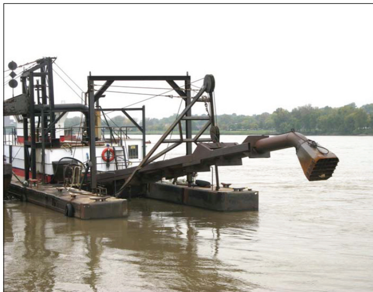
Figure 3. Suction-head dredge with elevated boom and suction head (USACE, 2011).
