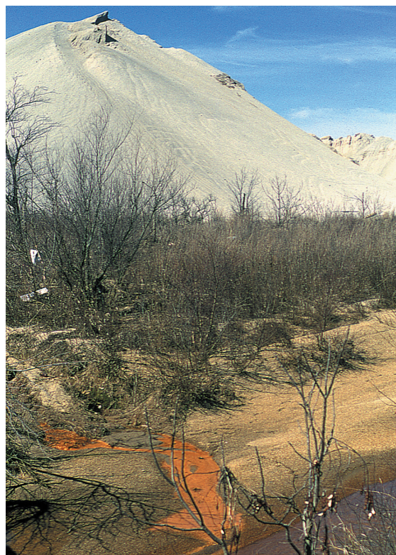
Figure 7. Water, contaminated by iron sulfide, flowing from tailing piles into Tar Creek near Picher, Oklahoma. The iron sulfide turns the water orange.
