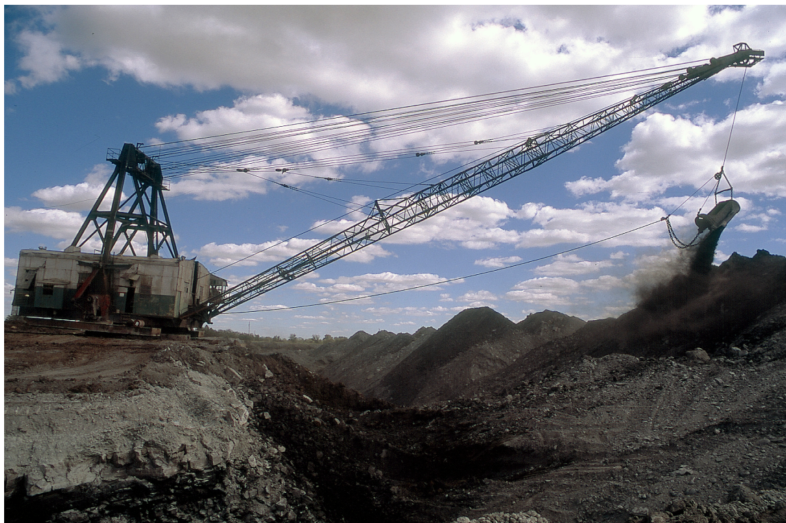
Figure 5. Coal strip mine in Crawford County using an electric shovel and dragline.
