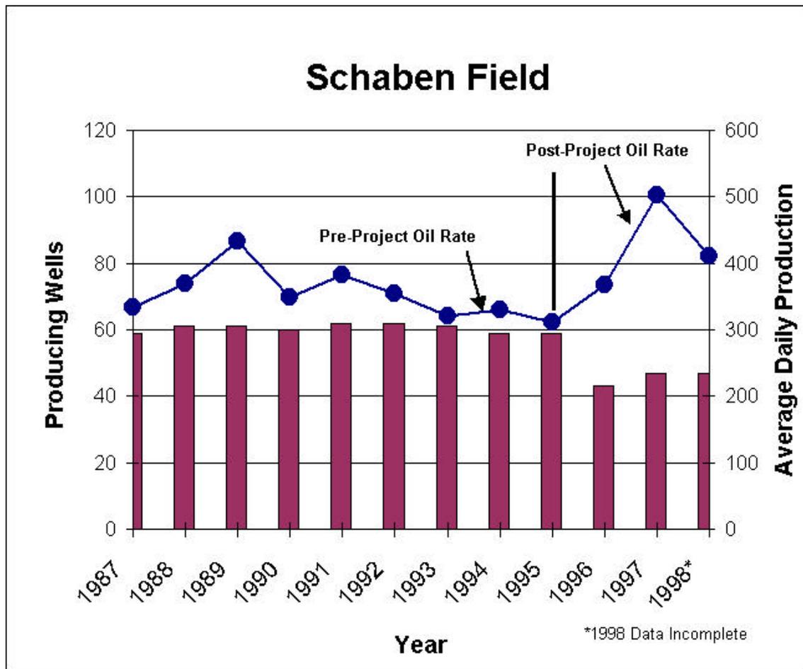
**Figure 1.** Average daily oil production rates for the Schaben Field Demonstration Site, Ness County Kansas. Producing rate from well has increased significantly as a result of targeted infill wells and recompletions.
