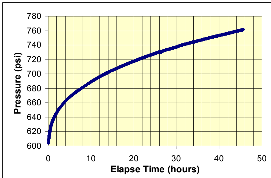
Figure 3. Bottom hole pressure build-up during water injection into Colliver #7 at a rate of 450 bbl/D (71.5 m 3 /d).
