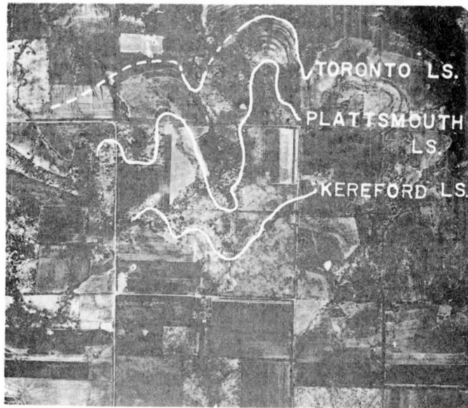
Figure 10. An aerial view of the outcrop pattern of the Oread Limestone Formation illustrating the proximity of the three limestone members that make up a large part of the construction materials resources in southeastern Osage County. Approximate scale, 1:24,000.
