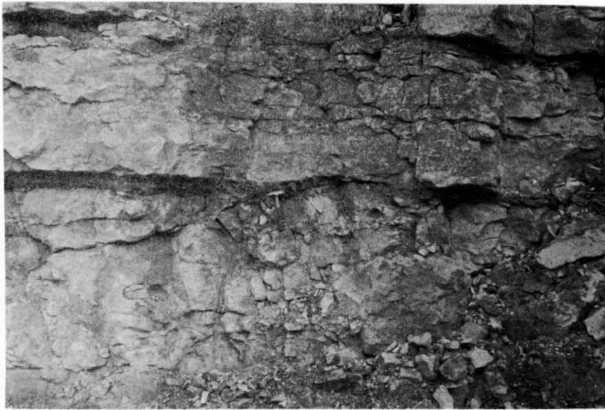
Figure 15. Quarry face of the Killough-Clark quarry which produces the Kereford Limestone for agricultural lime and aggregate for local use.
