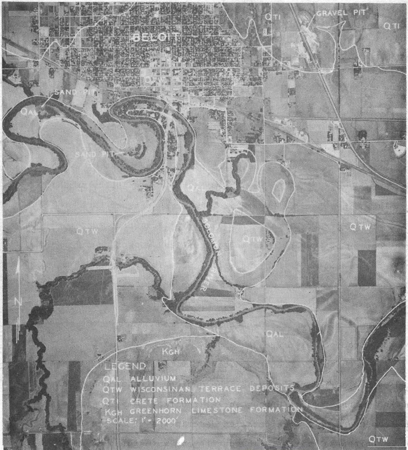
Figure 3. Three cycles of deposition in the Solomon River valley; Crete Formation, Wisconsinan Terrace Deposits, and Recent Alluvium. Sand and gravel pits in the Crete Formation and the Recent Alluvium are easily distinguished.
